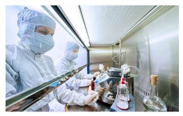
Gowned operator performing sterility testing in a laminar air flow hood
